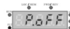
As illustrated 4-2, "p.oFF" is shown on electricity initialization of the electricity parameter display state.
