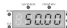
As illustrated 4-3, the setting frequency of stopping is shown "50.00" of the machine when stopped parameter display state
