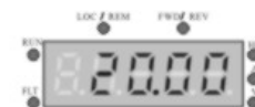
As Illustrated 4-4, output frequency when running shown by "20.00" on the running parameter display state
